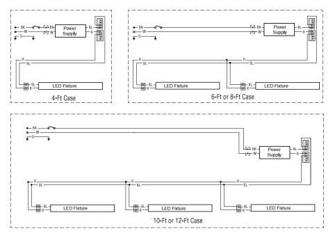
WARNING: All components must have mechanical ground, and the merchandiser must be grounded.
