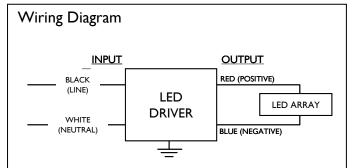
Input, Output and 0-10V Dimming use lead-wires. Lead-wires are 18AWG 105C/600V solid copper
